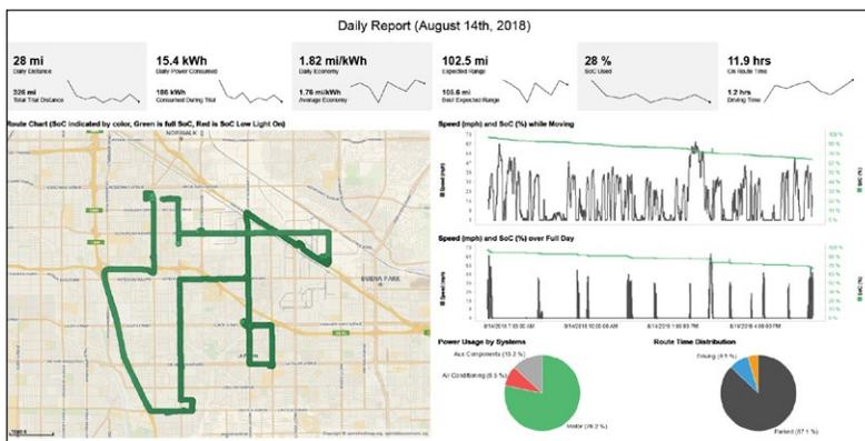
Lightning Analytics, our technical subscription service, goes much deeper than most commercial telematics solutions. By reporting GPS location and as many as 70 vehicle parameters every second over a 4G connection, a rich set of data on every vehicle's activities and status is collected.
